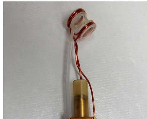
MIFEDs coil provide magnetic field strength and configuration
